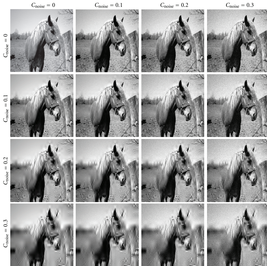
FIGURE 18: Images tested in [59] containing various combinations of structural distortion and additive white noise. The structural distortion was generated via quantization of wavelet subbands with per-subband distortions selected to disrupt global precedence as described in Section 5.1 (cf. Figure 9).
