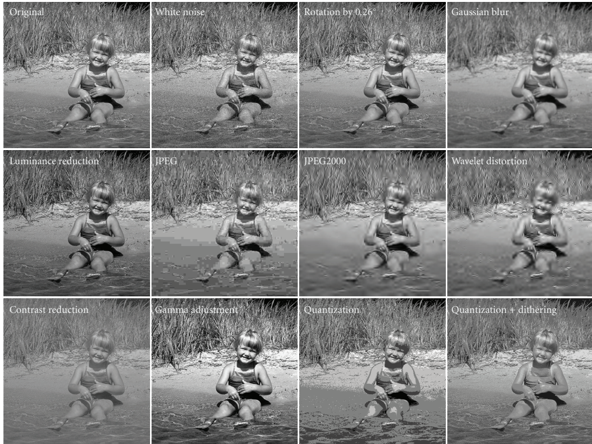
FIGURE 1: Original and distorted versions of the image child swimming from the CSIQ database [27]. Note the large variation in perceived quality, despite the fact that all distorted images have the same peak signal-to-noise ratio of 22.5 dB.
