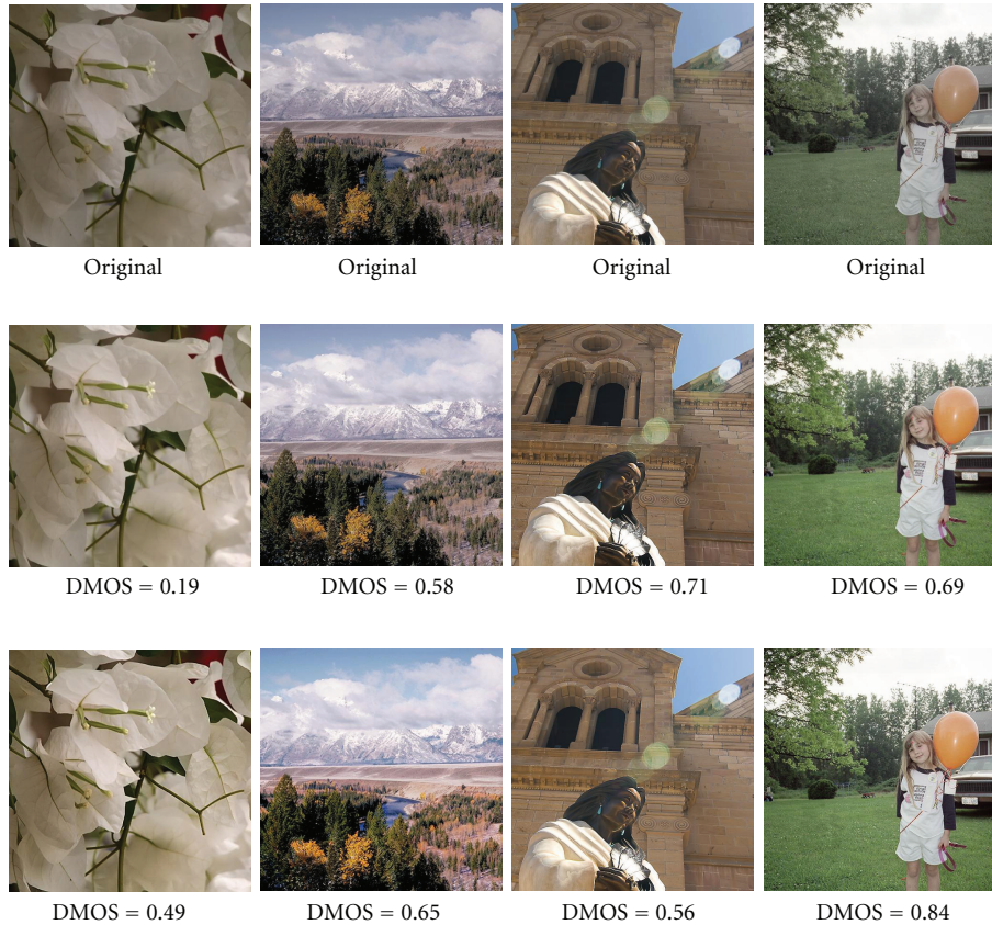
FIGURE 25: Examples of original and enhanced images from the DRIQ database [140, 341]. The DMOS values denote differences in perceived quality relative to each corresponding original and relative to all other enhanced images; larger DMOS denotes greater perceived quality.
