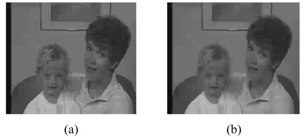
Fig. 17. H.264 decoded I-frame from Mother and Daughter video (QP = 42, \Delta = 80 ). (a) No filter (PSNR = 31.07 dB, PSNR-B = 28.64 dB, SSIM = 0.8232). (b) In-loop filter (PSNR = 31.39 dB, PSNR-B = 31.36 dB, SSIM = 0.8410).
