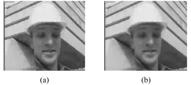
Fig. 16. H.264 decoded I-frame from Foreman video (QP = 42, \Delta = 80 ). (a) No filter (PSNR = 29.19 dB, PSNR-B = 26.63 dB, SSIM = 0.8041). (b) In-loop filter (PSNR = 29.71 dB, PSNR-B = 29.44 dB, SSIM = 0.8382).
