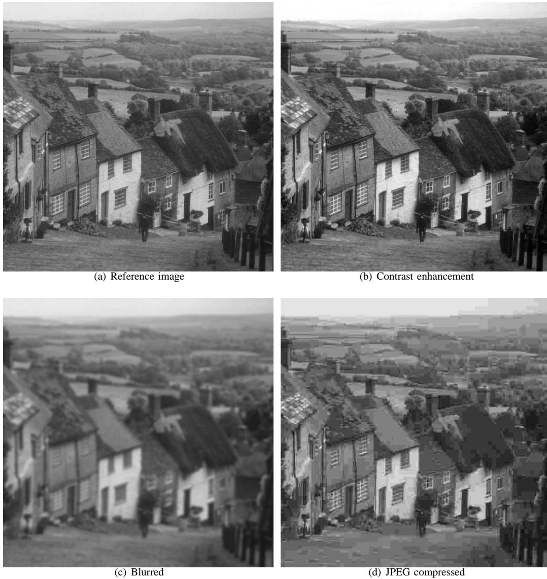
Fig. 6. The VIF has an interesting feature: it can capture the effects of linear contrast enhancements on images, and quantify the improvement in visual quality. A VIF value greater than unity indicates this improvement, while a VIF value less than unity signifies a loss of visual quality. (a) Reference Goldhill image (VIF = 1). (b) Contrast stretched Goldhill image (VIF = 1.10). (c) Gaussian blur (VIF = 0.07) and (d) JPEG compressed (VIF = 0.10).
