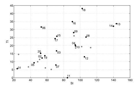
Figure 1. Spatial information (SI) and temporal information (TI) indicators<sup>20</sup> for all 30 sequences. The numbered dots represent the 20 sequences that have been selected for the experiment.
