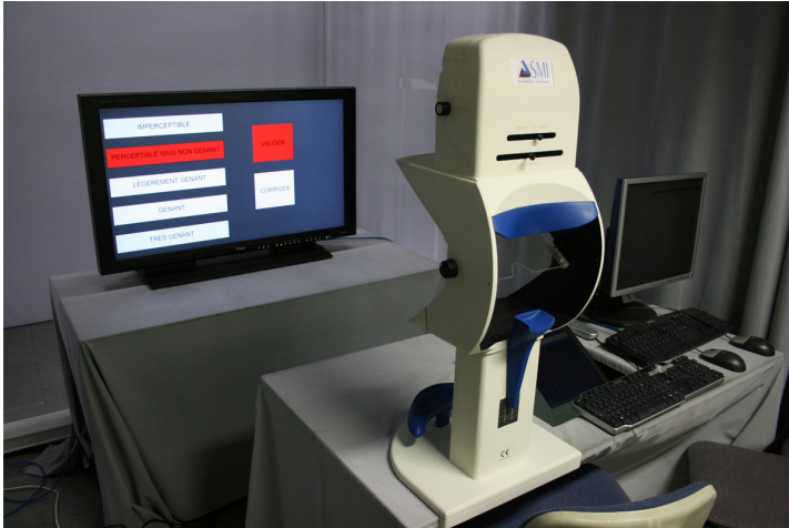
Figure 72: Laboratory setup with the SMI eye tracker in the foreground.
