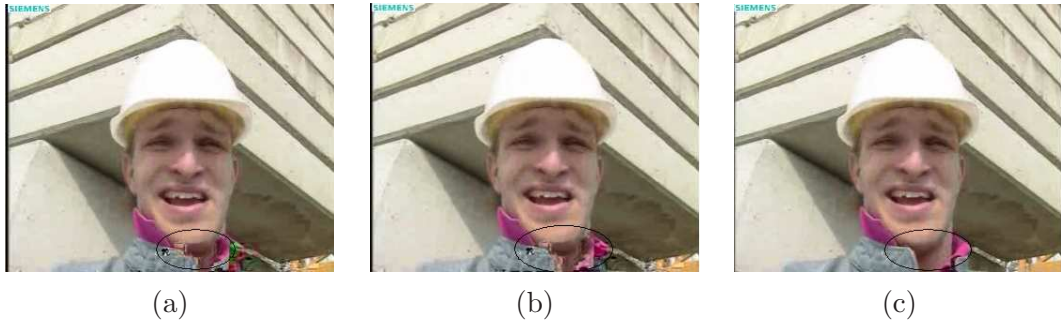
Figure 4.12: Difference in the two WEC algorithm implementations highlighted for Foreman video, frame 15, processed using H.264 for a packet loss of 0.6%: (a) No WEC, (b) I- in I-frame WEC, (c) P- in I-frame WEC.
