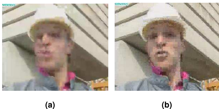
Figure 3.10: Artifacts introduced by (a) H.264 compression (blur effect) and (b) MPEG-2 compression (block effect)
