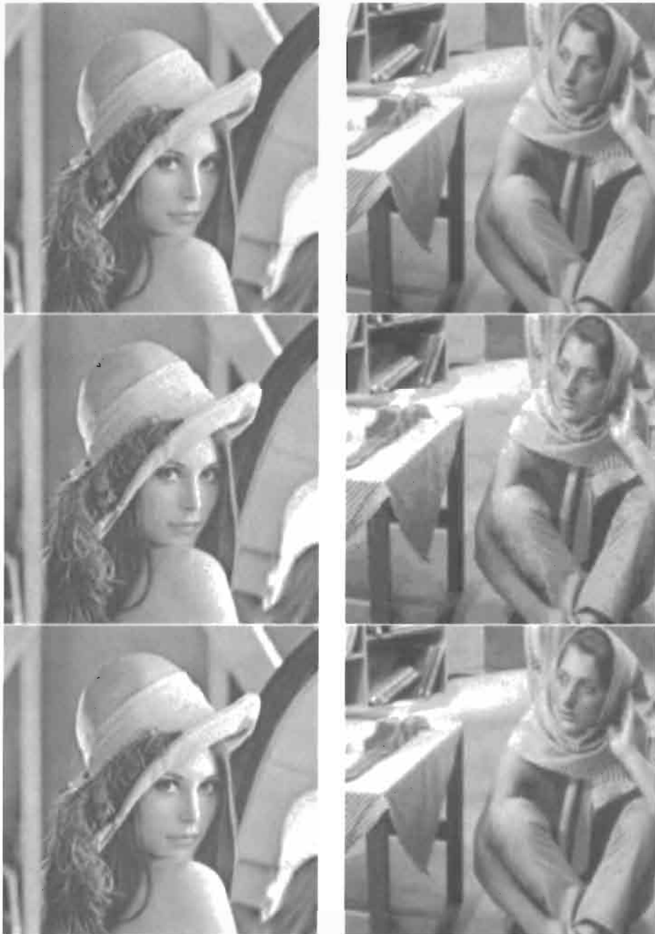
FIGURE 12 Coding of the 512 \times 512 Lena and Barbara images at 0.25 b/p (compression ratio of 32:1). Top: the original Lena and Barbara images. Middle: baseline JPEG decoded images, PSNR = 31.6 dB for Lena , and PSNR = 25.2 dB for Barbara . Bottom: SPIHT decoded images, PSNR = 34.1 dB for Lena , and PSNR = 27.6 dB for Barbara .
