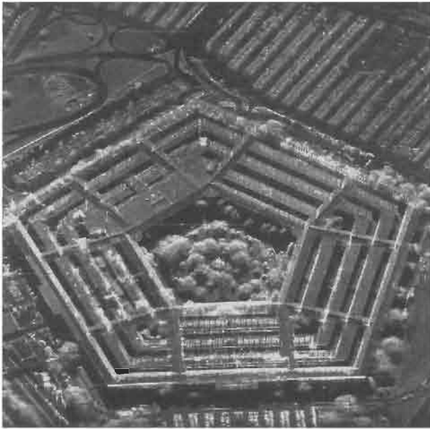
FIGURE 9 Spotlight mode X-band image of the Pentagon building, collected by the Data Collection System.
