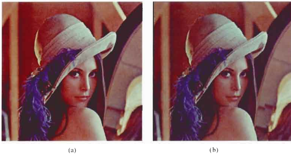
FIGURE 5.2.6 Illustration of the use of BTC in color image compression: left, original image; right, image encoded at 1.89 bpp.
