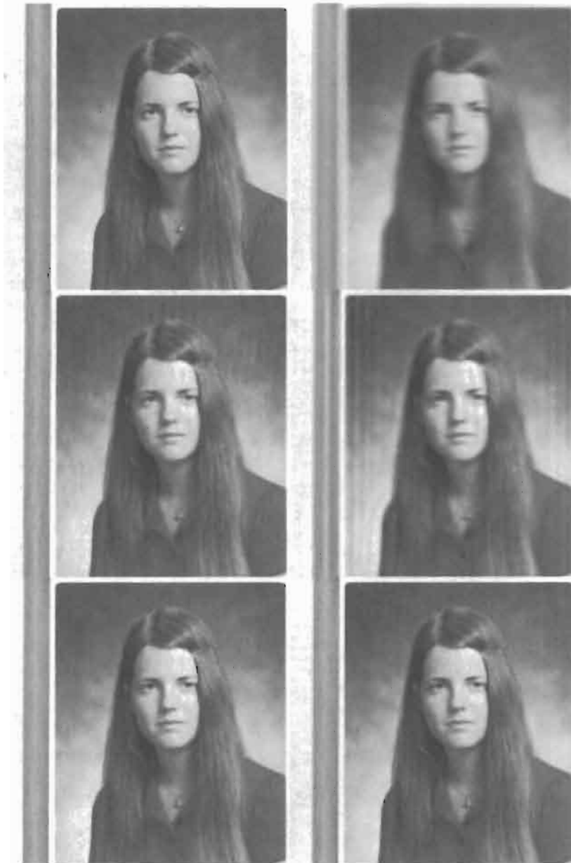
FIGURE 2 Example of a multichannel LMMSE restoration: original (upper left), degraded (upper right), restored single-channel statistics obtained from original (middle left), restored single-channel statistics obtained from degraded original (middle right), restored multichannel statistics obtained from original (lower left), restored multichannel statistics obtained from degraded (lower right). (See color section, p. C-6.)
