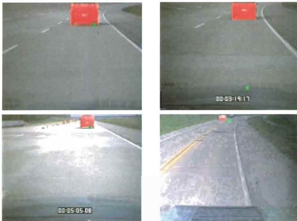
FIGURE 4.7.5 Correct estimation of the vehicle ahead, using the MAP procedure.
