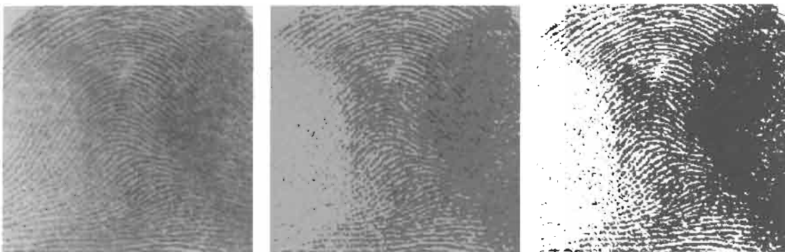
FIGURE 10 Quantization of the 256 \times 256 image "fingerprint." Clockwise from left: 4, 2, and 1 bits per pixel.
