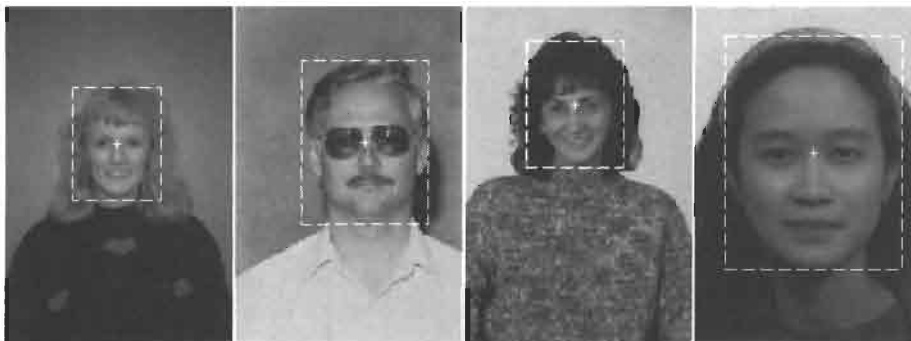
FIGURE 6 Examples of multiscale face detection.
