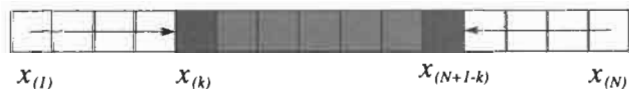
FIGURE 4 CWM smoothing operation. The center observation sample is mapped to the order statistic x_{(k)} ( x_{(N+1-k)} ) if the center sample is less (greater) than x_{(k)} ( x_{(N+1-k)} ) and left unaltered otherwise.
