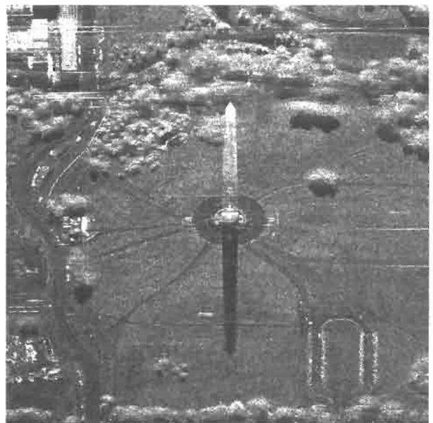
FIGURE 8 Spotlight mode X-band image of the Washington Monument, collected by the Data Collection System.
