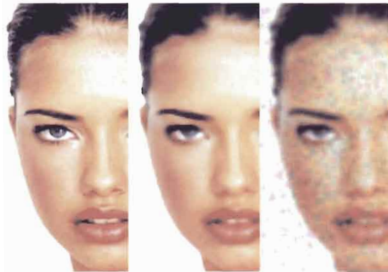
FIGURE 3.2.11 (Enlarged) Noise-free image (left), 5 \times 5 median smoother output (center), and 5 \times 5 mean smoother (right).
