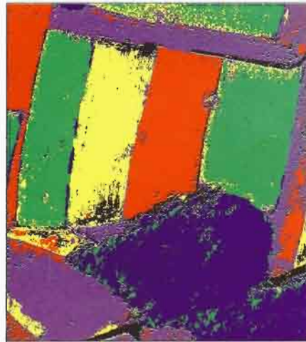
FIGURE 4.7.8 Segmentation of another aerial image, this time of a rural crop field area, using the same texture-based maximum likelihood procedure employed in Fig. 7.
