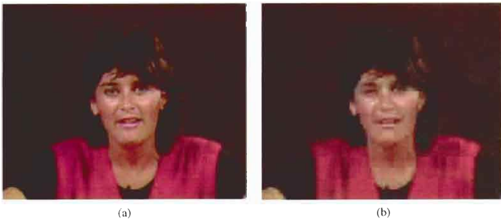
FIGURE 6.1.4 Severe blocking artifacts introduced by gross quantization of DCT coefficients: (a) original, (b) reconstructed.
