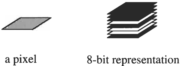
FIGURE 9 Illustration of an 8-bit representation of a quantized pixel.
