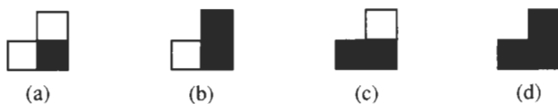
FIGURE 8 Pixel neighbor relationships used in a region labeling algorithm. In each of (a)–(d), f(\mathbf{n}) is the lower right pixel.
